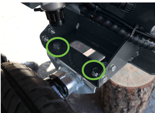
2 bolts and nuts on each side with torque of 72-76nm
