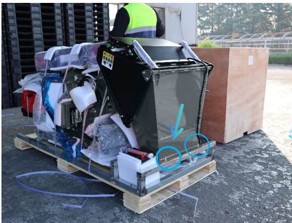
Attention: Disassemble these two bolts before moving feeding hopper
