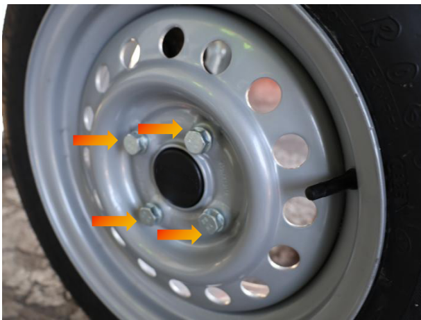
4 bolts on each tire with torque of 90-100nm , presure 32-36 psi
