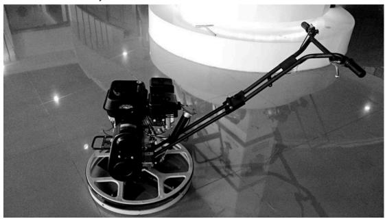
Machine is heavy and awkward to move around. Use proper heavy lifting procedures and DO NOT LIFT THE MACHINE BY GUARD RINGS.
