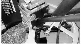
4. Remove bolts from adjusting cable, connect cable to knock pin and fasten the bolts.
