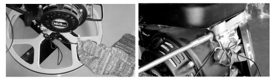
6. Fix engine stop cable (also from handle pipe) to engine by three-way tube.
