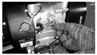
7. Fasten connect screw of handle and tie all cables by ribbon.
