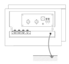
If it is D grounding (No.3 grounding), the grounding resistance should be lower than 100  $\Omega$ . When the voltage is over 300V, it is C class grounding and the grounding resistance must be lower than  $10\Omega$ .
