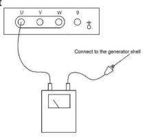
insulation resistance between the output terminal and the generator frame.
