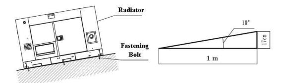
(7) There must be enough room around the genset for cooling and maintenance. Keep the genset at least 1 meter away from walls and 2 meters away from the ceiling. Keep the air outlet and exhaust vented upwards and prevent any blockage. This will help prevent overheating and poor engine performance due to excessive back pressure.
