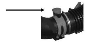
5. Remove the rubber cover from the collector.
