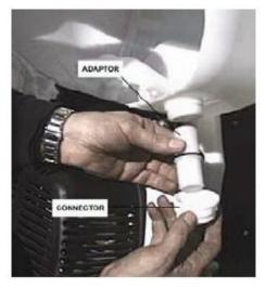
3. Install the duster adapter into the tank (please remember to install the O-ring correctly). Insert the air distributor into the tank (install with the connector).
