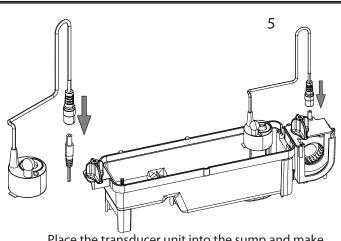
Place the transducer unit into the sump and make the connection
